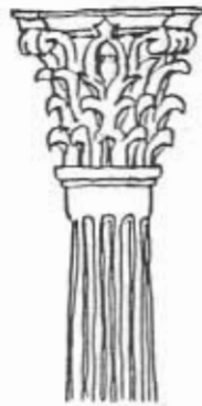
CAST IRON COLUMN
